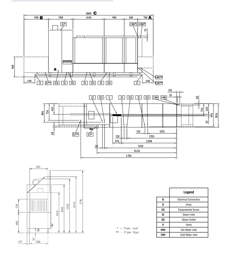
For different loading zone (A), unloading zone (B) and total length (C), please refer to the loading and unloading zone table on the last page.
